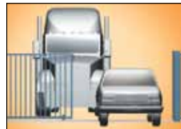
partial open allows long gates to open 14 feet for automobile traffic, or opens gate fully for large trucks or oversized vans
