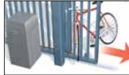
entrapment prevention system reverses gate on contact
